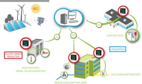
• MEASUREMENT OF WATER, HEAT, GAS ETC. CONSUMPTION VIA PULSE INPUTS
