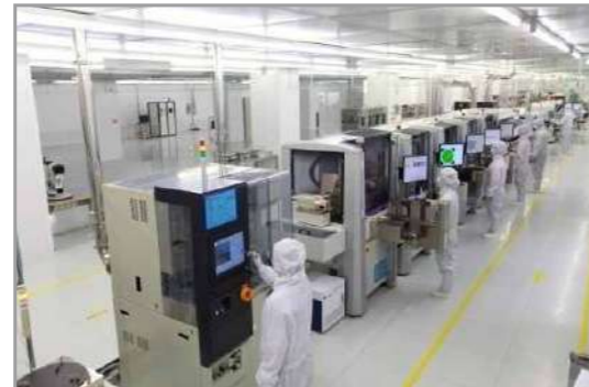
IGBT module automatic packaging line
