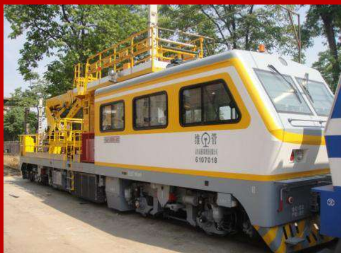
JZW-4G OCS Aerial Maintenance Vehicle
