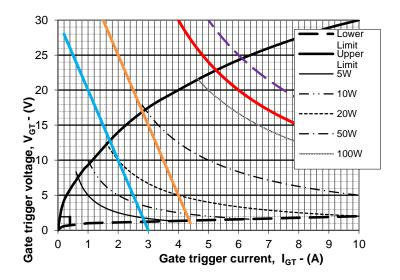
The load line is then compared to the 150W curve or the power calculated from the values of current and voltage where the load line intercepts the upper gate characteristic at 2.8A and 17 i.e. 48W. Either way our initial gate pulse is less than 150W and our gate drive is fully acceptable from a gate power point of view.
