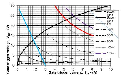
Therefore our gate drive complies with the limit of 120W when connected to our thyristor.
