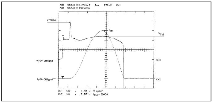
Fig. 7 Example of high spike voltage
