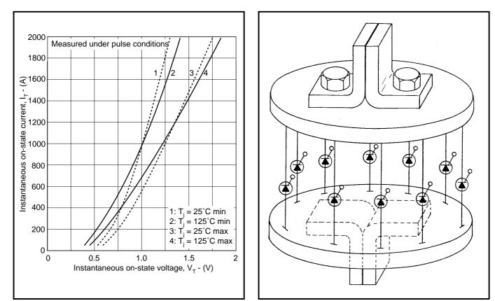
Fig. 2 Thyristor limit on-state characteristics
